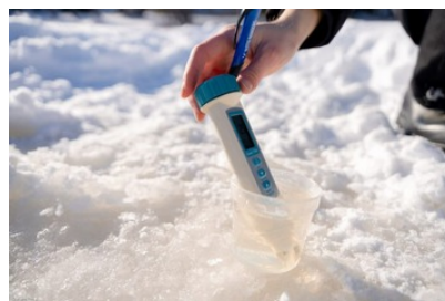
The Winter Chloride Watchers test kit makes it easy to monitor local waterways for excess chlorides.
